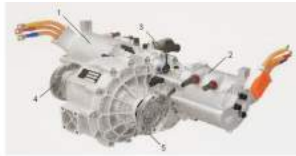
Figure 27 Driven by two transverse engine. 1,2 - liquid-cooled AC motors; gear shift mechanism; 4,5 - differential axles
