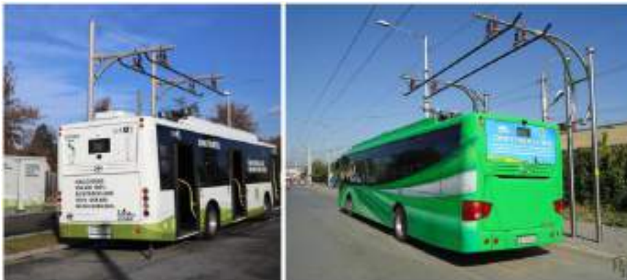
Figure 18 Supercapacitor e-buses (Chariot) on charging station in Graz and in Sofia.
