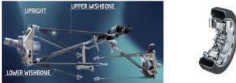
Figure 30 Suspension of a Formula E car 63 and mounting a motor in the wheel
