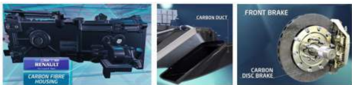
Figure 26 Use of carbon to lighten the racing assembly units
